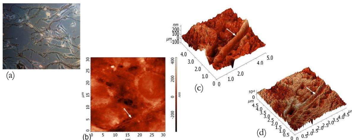
Fig.2 (a) Optical microscope image of complex structures made of cells and CNTs; (b) AFM image of such structures; (c) AFM detail of the previous image; (d) SMM image of the same detail. The latter image highlights features completely different from topography (c). These are ascribed to material dielectric contrast.
