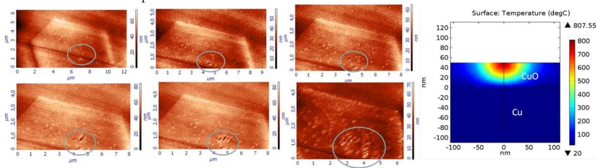
Fig.4 Consecutive scans of a graphene island on copper substrate, after localized microwave exposure through SMM tip (*left*). Each exposure generates a new hole on the surface. The process is highly controllable. COMSOL simulation: thermal gradient due to microwave localization (*hot spot*) (*right*).
