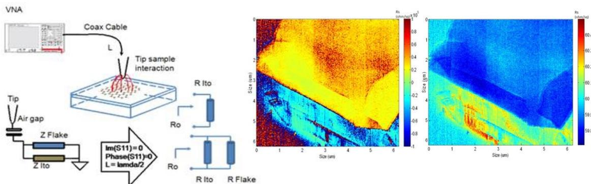
Fig.1 Schematic description of the lumped element circuit used to model the SMM interaction with graphene+ITO multi-layered sample. The approximation is valid only when the conditions in the arrow are satisfied (left). Maps of the spatial distribution of sheet resistance; graphene only (centre) and graphene+ITO case (right).
