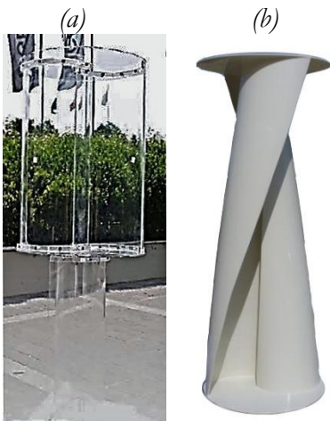
Figure 6: Constructed prototypes of Savonius rotors: (a) two-stage straight and (b) helical configurations.
